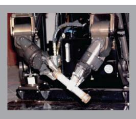
US Air Force "ARTS" vehicle, equipped with dual Raptor force feedback manipulator arms for the remote handling of unexploded ordnance.
