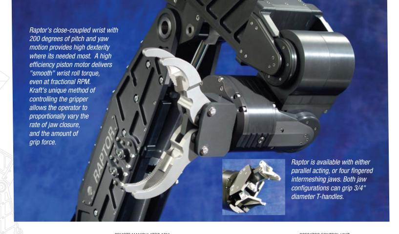
Raptor requires only one electrical connection and a pressure & return hydraulic connection. All valves are packaged as an integral part of the manipulator arm, eliminating the cumbersome hydraulic lines that would be necessary with a remote valve package. A square, four-bolt flange makes mounting the arm simple.
