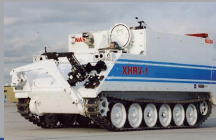
An experimental NASA HazMat vehicle equipped with a Grips manipulator arm to assist emergency personnel while responding to a chemical, biological or radiological threat.
