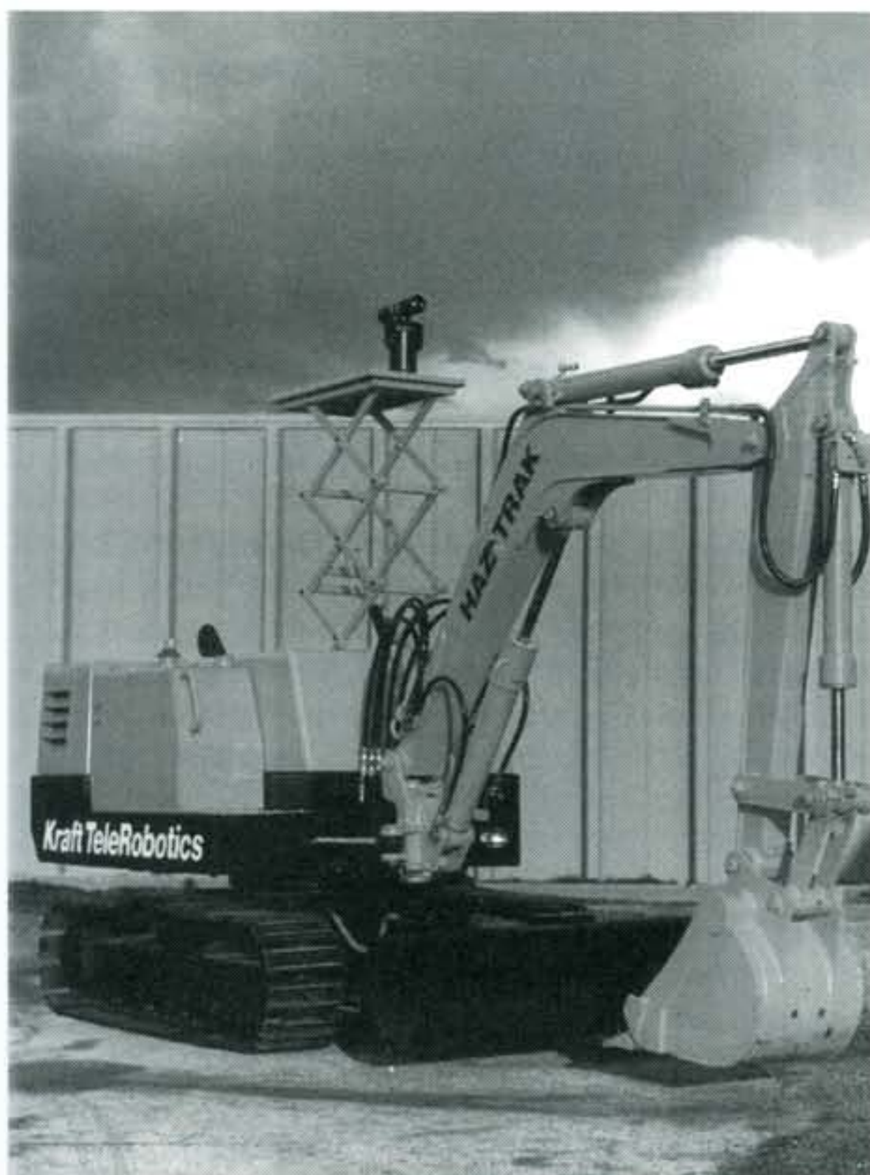
Unlike an excavator operator, the manipulator operator is intuitively linked to the arm he is controlling through a single hand controller that is responding to his own natural arm motion.
