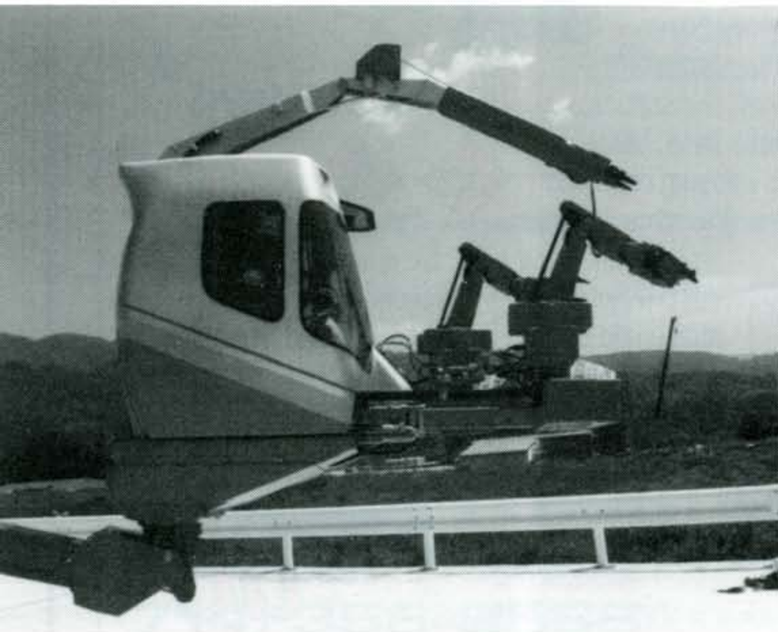
Unlike an industrial robot, a telerobotic system responds to the direct commands of a human operator.
