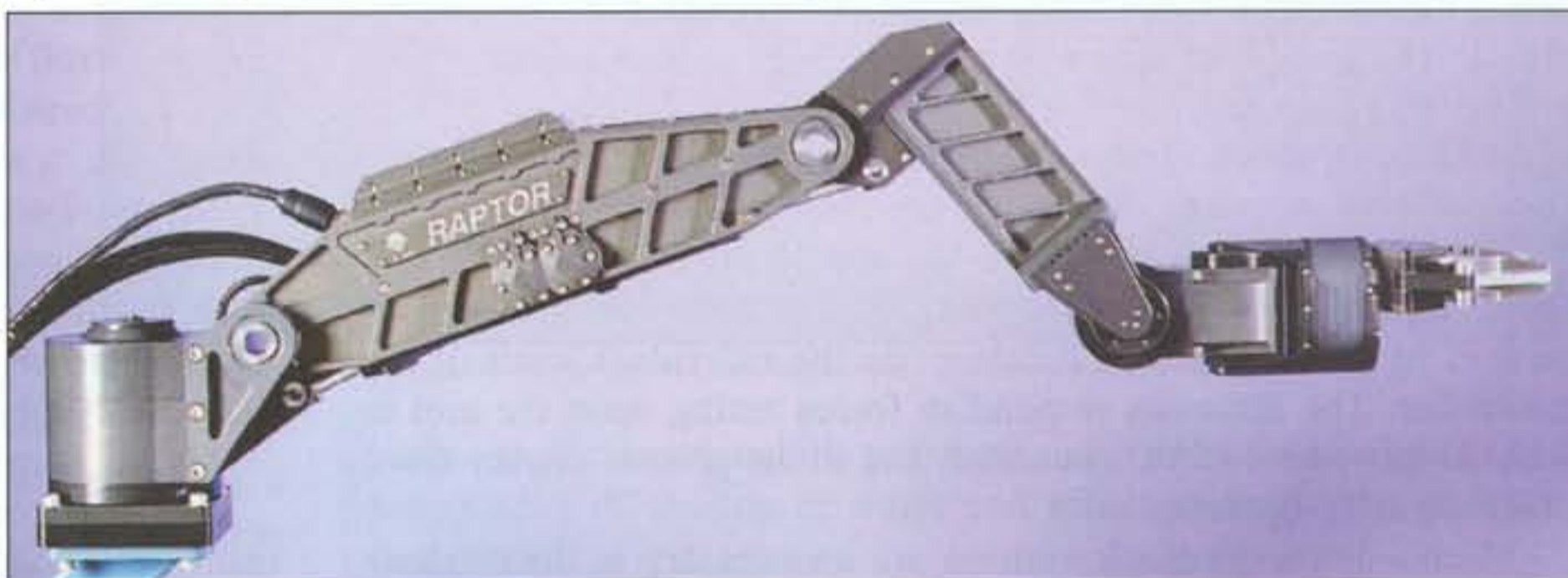
Kraft's Raptor offers the option of force feedback, allowing the operator to feel the movement of the arm underwater.
