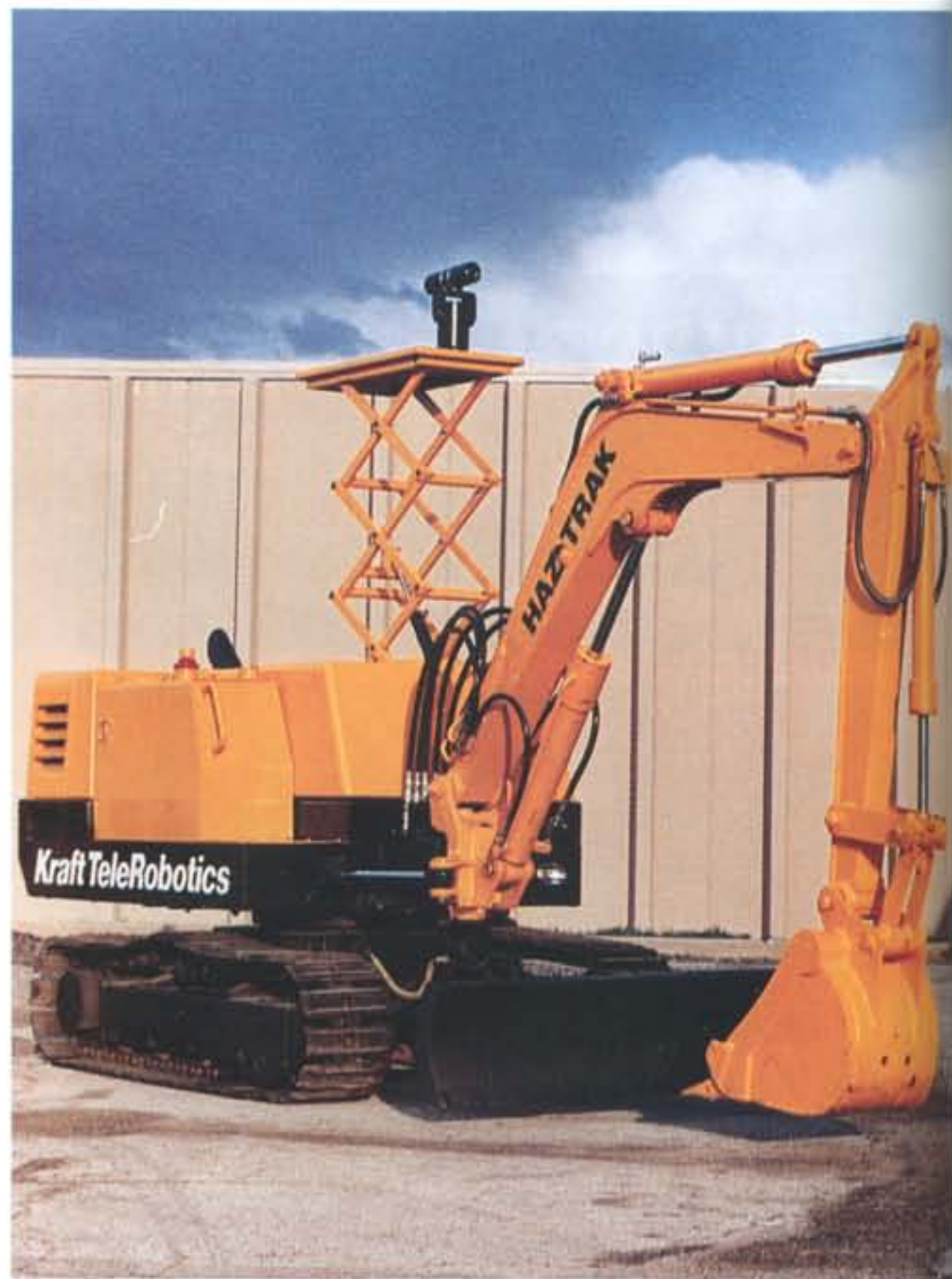
Haz-Trak, a force feedback telerobotic excavator developed by Kraft Telerobotics, Inc.
