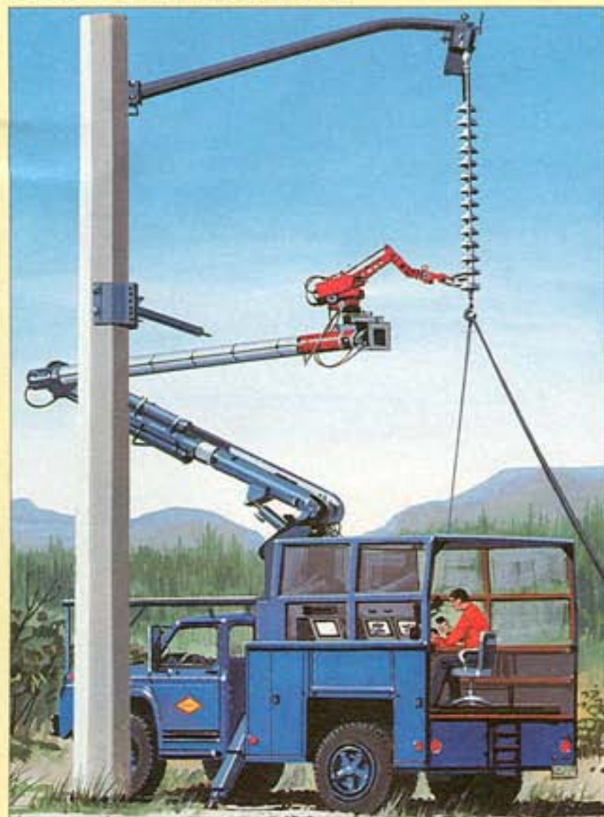
Safe in his truck, a teleoperator repairs line by remote control.
