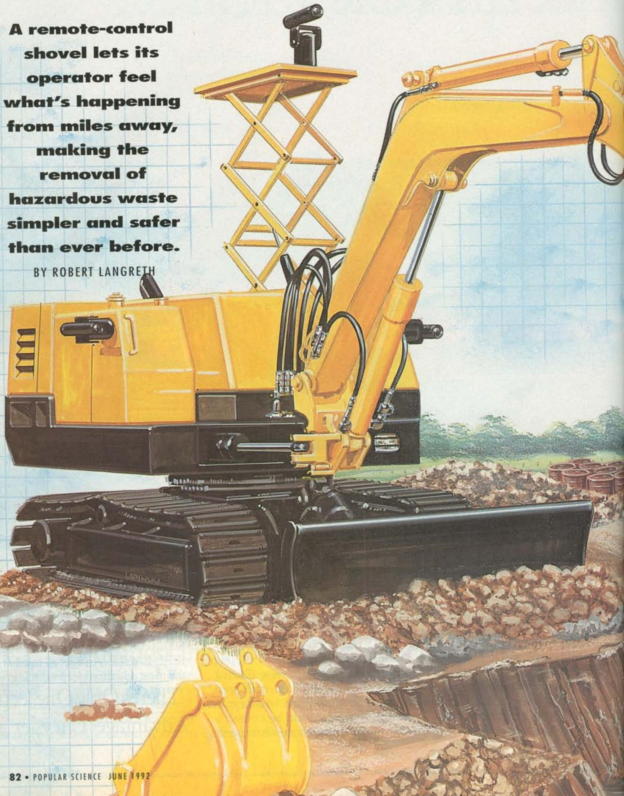
**P**erched in the middle of a radioactive waste site, the giant yellow machine looks like an ordinary hydraulic excavator, except there is no operator, or place for an operator. The only sign that humans might be watching are three cameras mounted on a platform above the engine.
