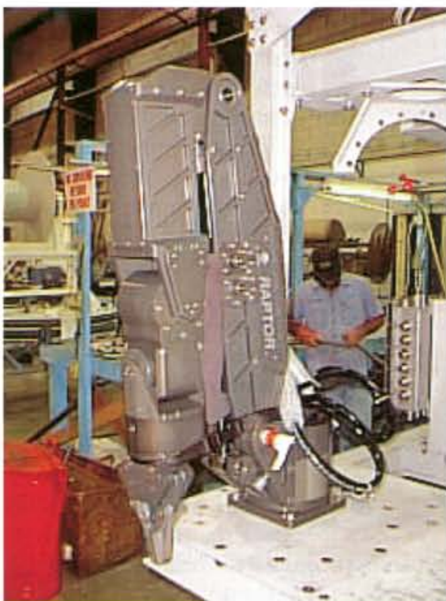
Kraft manipulator will turn Terra Nova's knobs
