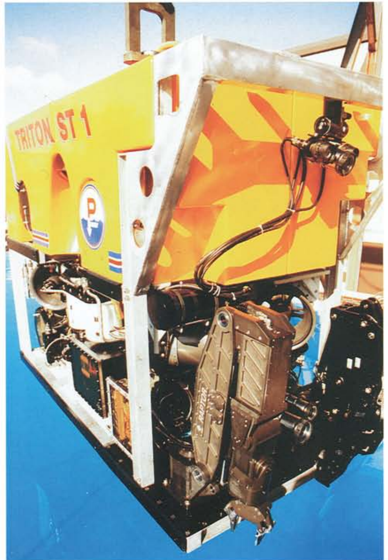
Force Feedback Raptor on Ceanic's New Triton ST. Ceanic Currently Has 7 Force Feedback Raptor Arms on Order
