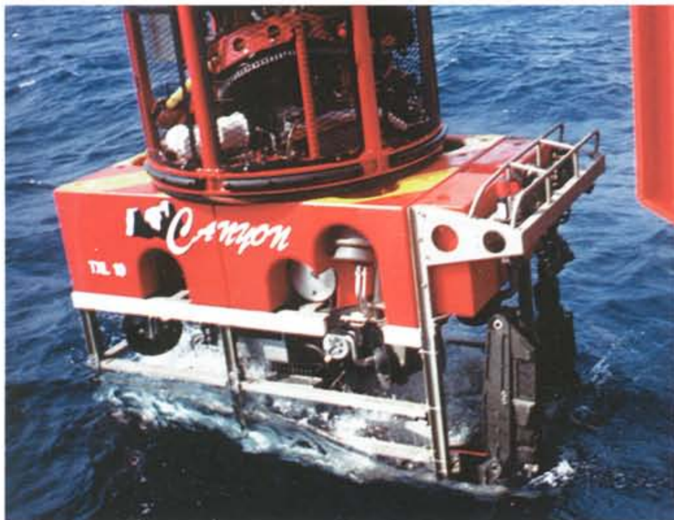
Predator Arm on Canyon Offshore ROV
