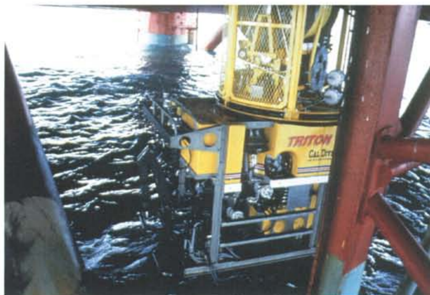
Cal Dive ROV operating with the Predator Arm
