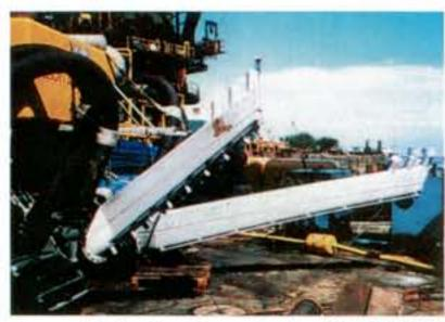
Purpose-built plough attached to FLEXJET II
