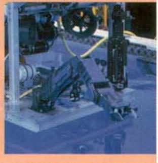
completion of remote work tasks in the deep ocean, and hazardous inland environments. Constructed primarily of anodized aluminum and stainless steel, it is rugged, reliable and completely field serviceable. It has a dry weight of 160 lb., wet weight of 98 lb., an 80-in. reach and lift capacity of 200 lb. at full extension. PREDATOR is priced at \$119,000 complete. Call (913) 894 9022 or fax (913) 894 1363.
