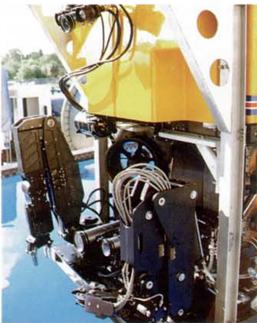
Kraft 7-function Raptor SC arm and ISE 7-function Magnum arm on a 10,000 ft. Perry Triton ST
