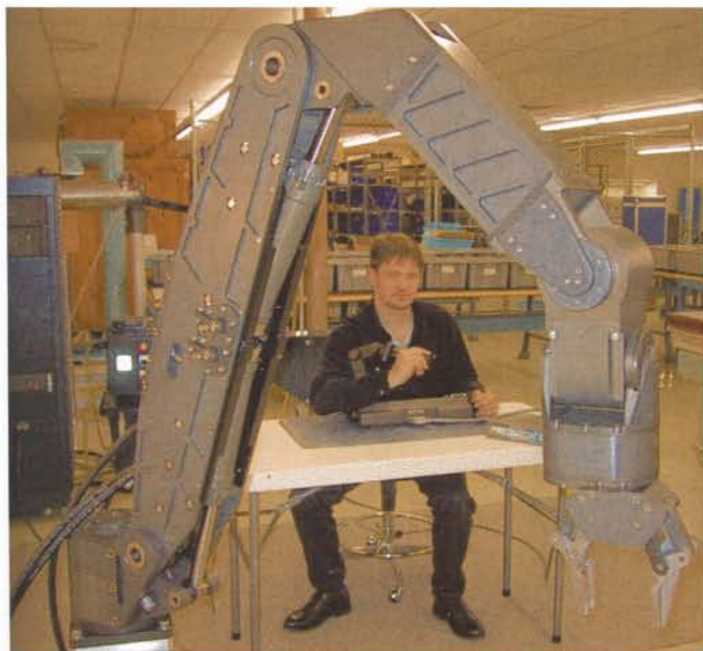
Mini-master in hand, Mr. Bernd Ocic of Ocean Frontier Services takes control of a new Kraft Predator II force feedback manipulator.
