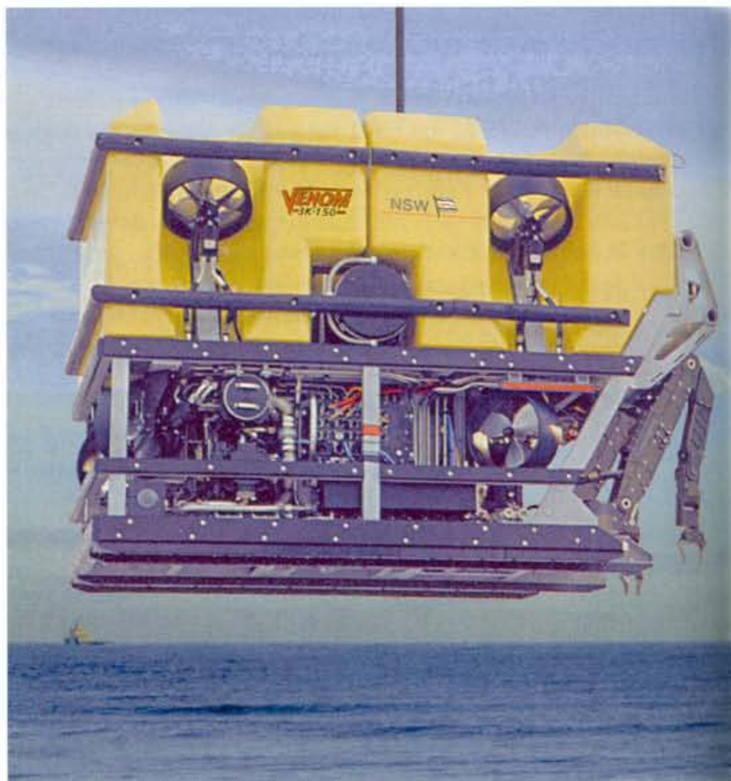
Hydrovision Venom ROV equipped with two Kraft Predator II force feedback manipulator arms
