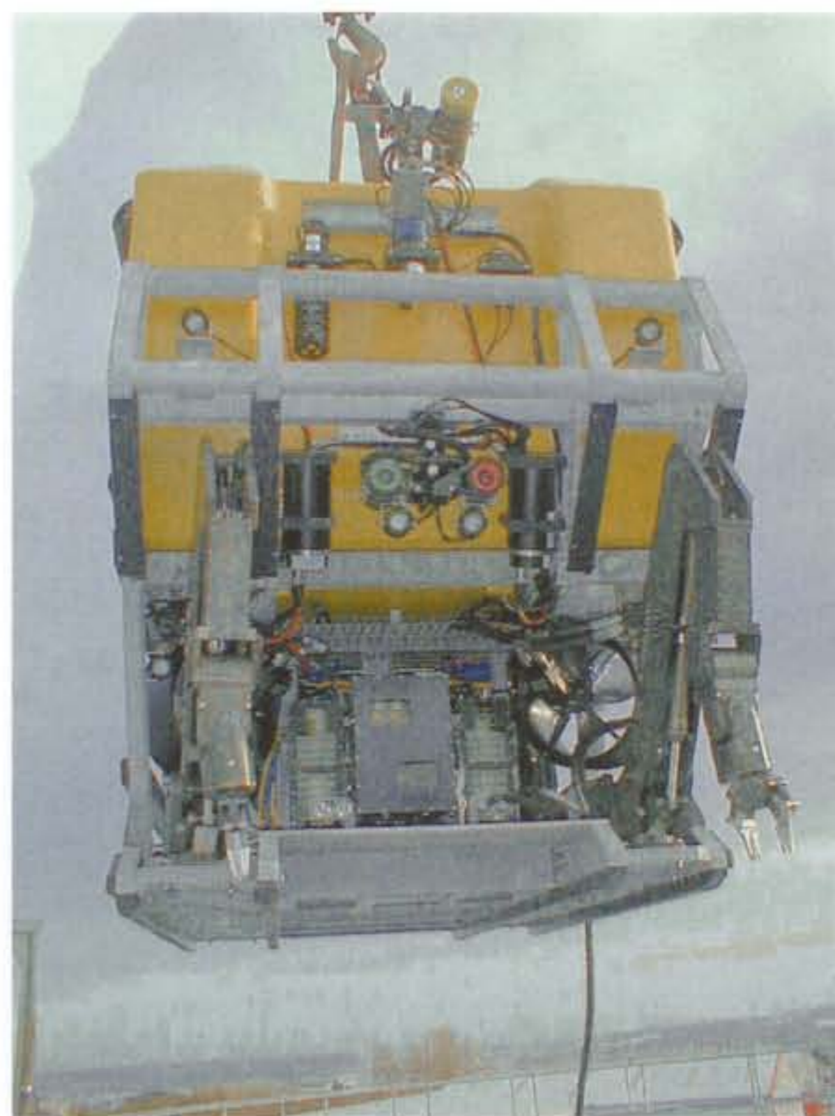
Front view of Venom ROV with Predator IIs
