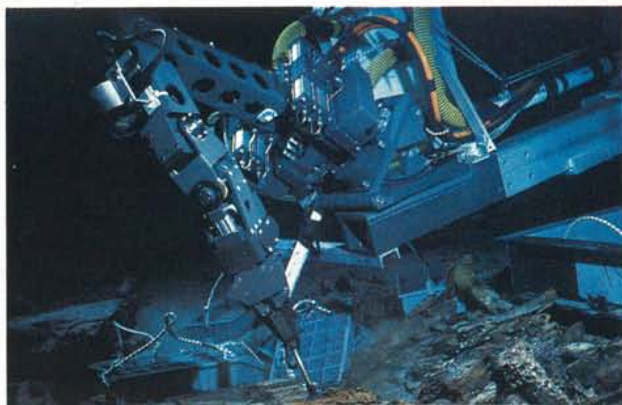
Undersea robot Nemo is the size of a truck and weighs 12,000 pounds.
