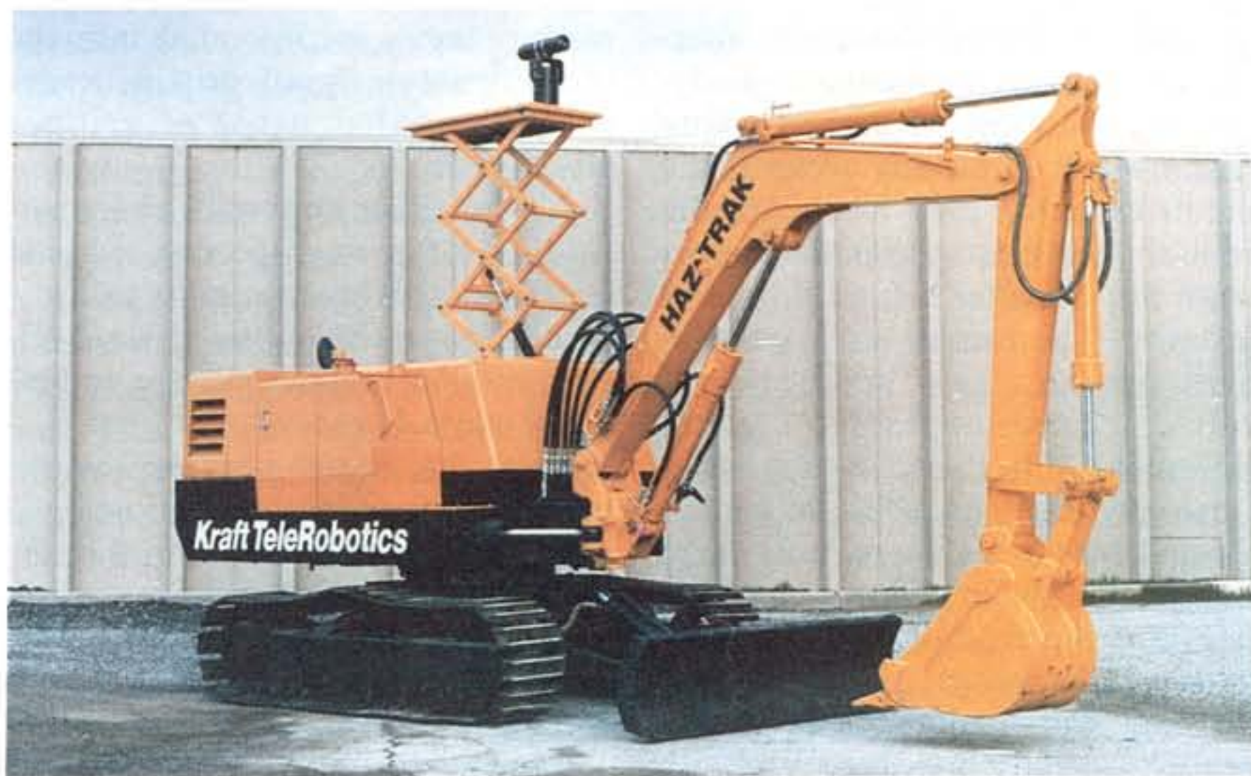
Telerobotic Haz-Trak system remotely controls downsized, 6800-lb excavator with maximum digging radius of 15 ft, 5 in., that can travel at speeds to 2 mph.
