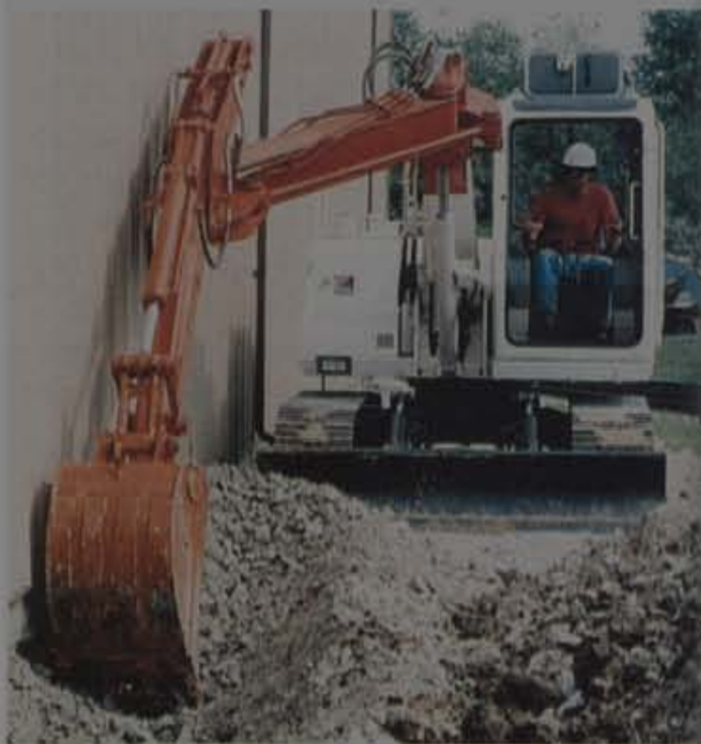
Boom-offset cylinder is pinned between lugs on base section and tip section of 3-piece boom on side outboard from operator. Offset rod — seen along operator's side of boom midsection — pins between same two attachment points on opposite side of boom.
