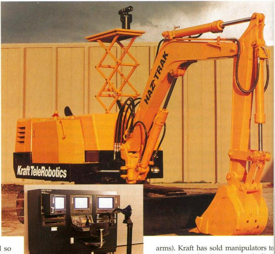
Kraft TeleRobotics' Haz-Trak is a remotecontrolled excavator that can be controlled up to one mile away with the console. As the operator moves the controller (shown right of the chair), the boom and bucket will move in the same manner.
